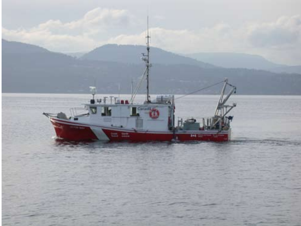
Figure 26. CCGS Otter Bay showing A-frame and working deck for deploying sampling gear. Source: Canadian Hydrographic Service.
