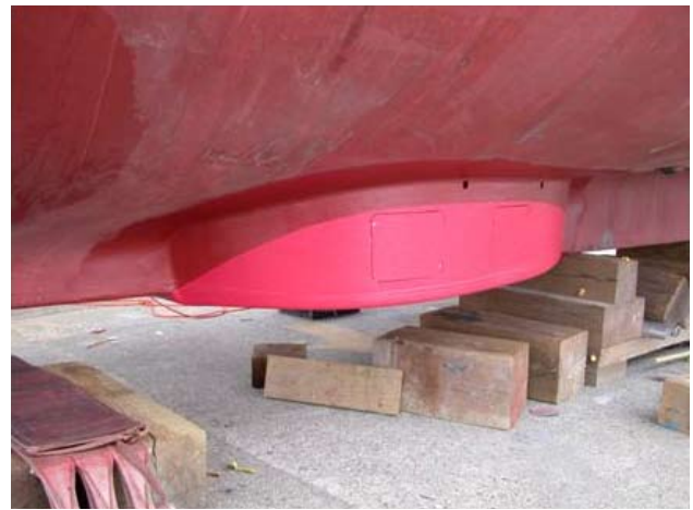
Figure 11. Half of pod (fairing) that protects along-keel transducer frame. Credit: Ocean Mapping Group, University of New Brunswick.
