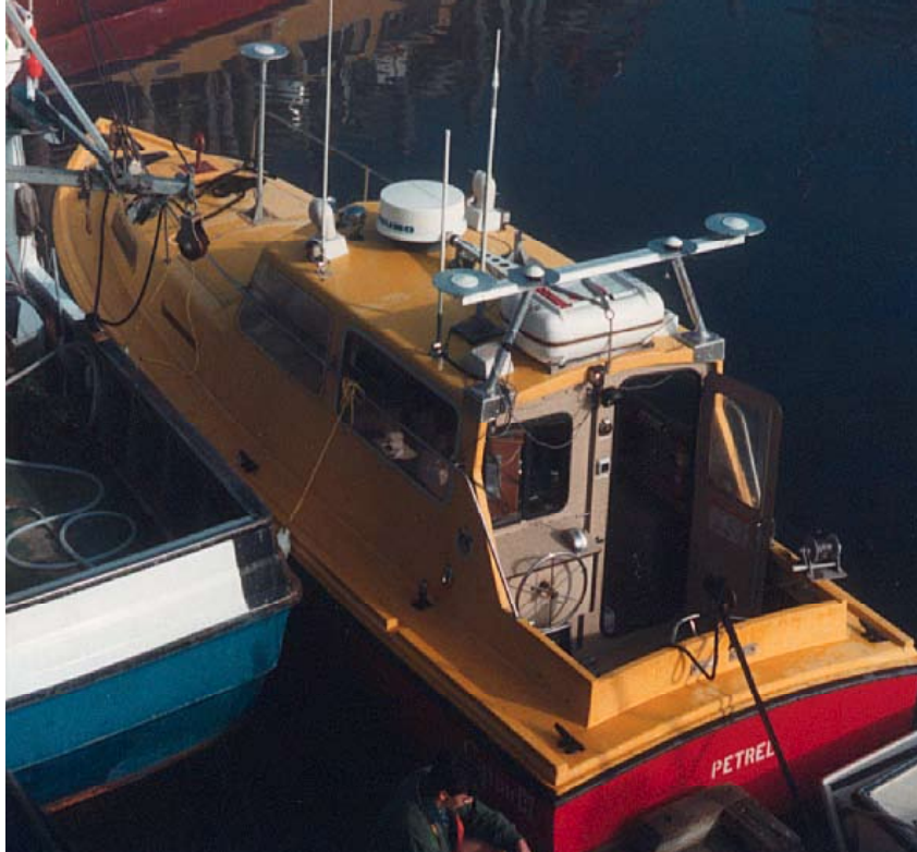
Figure 21. Typical launch installation of positioning, navigation, communications, and safety equipment. Credit: Andre Godin, Canadian Hydrographic Service.
