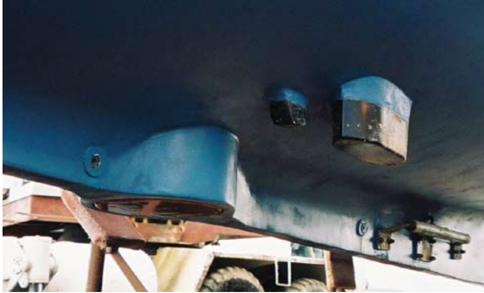
Figure 9. Examples of in-keel fairing, prone mounts, and debris cutters. Credit: Ocean Mapping Group, University of New Brunswick.
