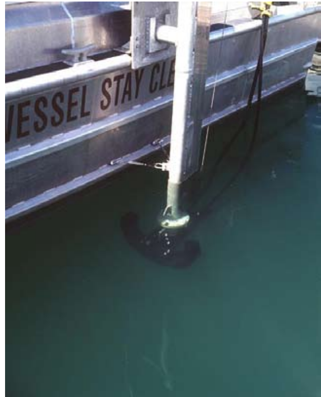
Figure 14. Example of over-the-side pole-mount installation. Source: Canadian Hydrographic Service.
