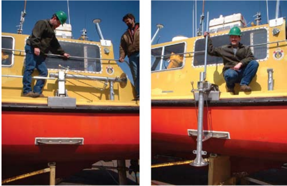
Figure 16. Permanent OTS transducer mount for new sensor testing (left = deployed; right = stowed). University of New Brunswick Ocean Mapping Group vessel Heron .
