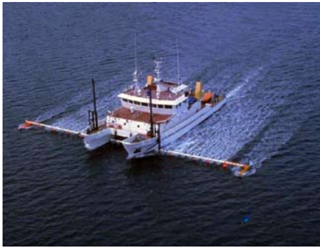
Figure 3. FCG Smith Sweep vessel (33 SBES transducers). Source: Canadian Hydrographic Service.
