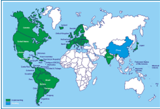
Figure 22. Coverage of SBAS, active and proposed. Green: North American WAAS, European EGNOS, Japanese MSAS (or MTSAS), and proposed Indian GAGAN. Blue: proposed Chinese system. White: no SBAS coverage. Source: Federal Aviation Administration.
