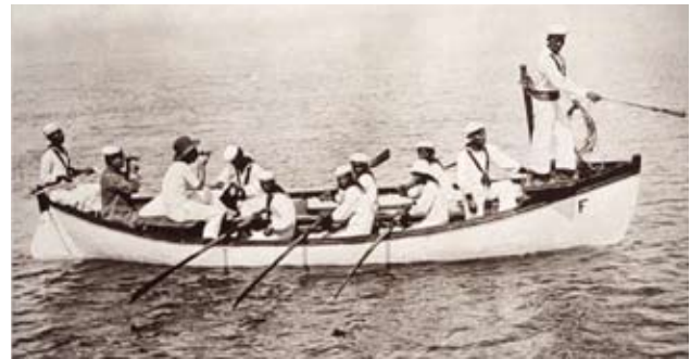
Figure 1. Swinging the lead. Note two gentlemen near the stern, each with a sextant and a notekeeper just ahead of them. Source: NOAA Photo Library.
