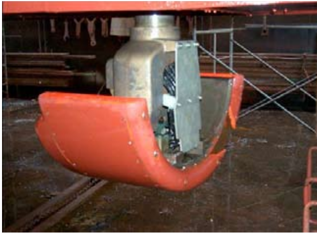
Figure 18. Transducer deployed below watertight well showing log damage to leading edge. Source: Canadian Hydrographic Service.
