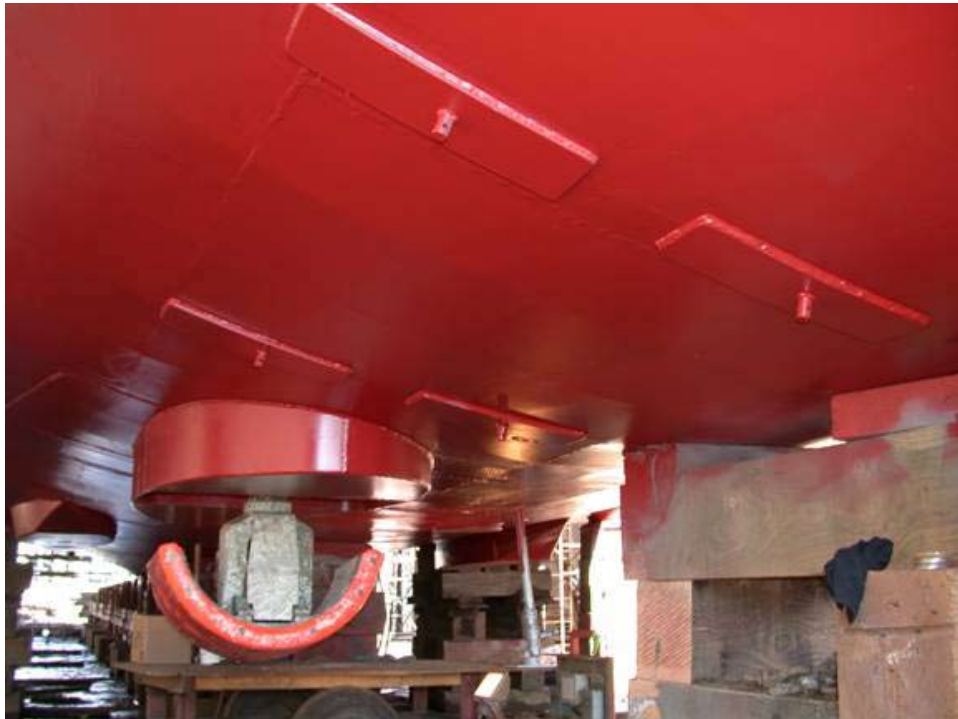
Figure 17. EM1002 transducer deployed below hull on ram. When retrieved, it lies inside a watertight well. Source: Canadian Hydrographic Service.
