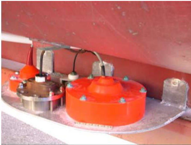
Figure 10. Three transducers mounted in a frame alongside keel. Source: Canadian Hydrographic Service.
