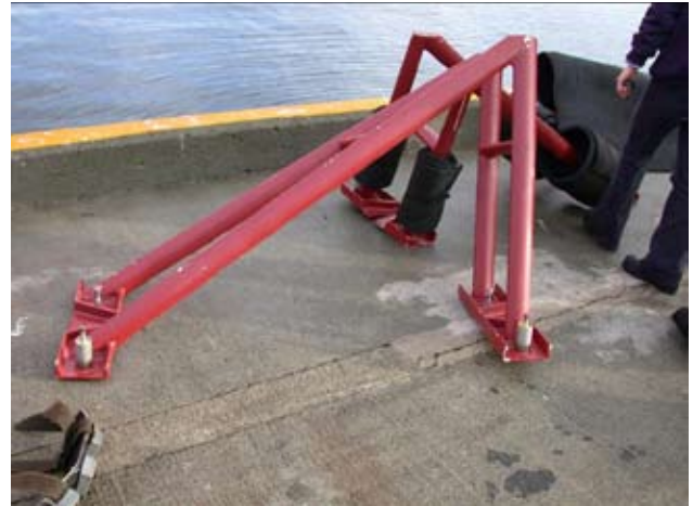
Figure 19. Transducer protection grids that attach to pins shown in Fig. 17. Source: Canadian Hydrographic Service.
