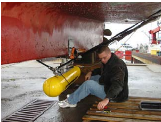
Figure 13. Keel-mounted Benthos C3D BSSS (straps and cabling run outside hull). Source: Canadian Hydrographic Service.
