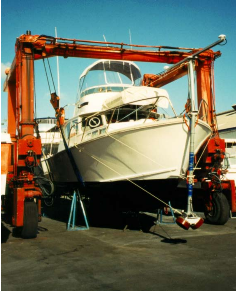
Figure 15. Example of over-the-bow pole-mount installation. Source: Canadian Hydrographic Service.
