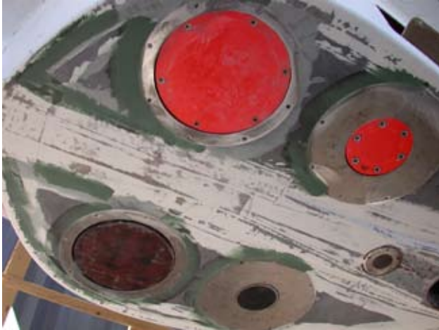
Figure 12. View of transducers in pod from below, showing both sides of the keel. Source: Canadian Hydrographic Service.
