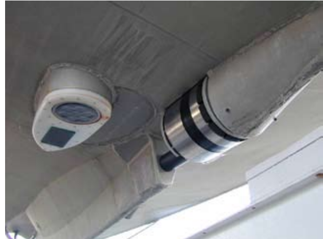
Figure 8. Examples of fairing and prone transducer mounts. Credit: G. Noll, NOAA.
