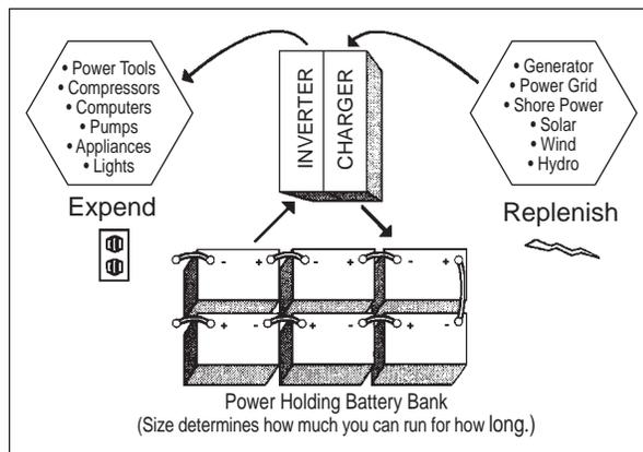
Inverters can convert 12-volt direct current from batteries to 120-volt alternating current, providing power to appliances, tools, and computers on board. Illustration shows simple diagram of the inverter cycle.
